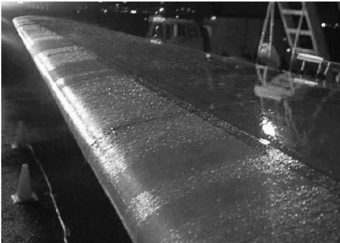
FIGURE 04 - FAILED TYPE IV ANTI-ICING FLUID BANDS
